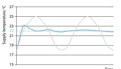
Variable speed compressors are designed in VERSO units. The major benefit of this type of compressor is it's flexibility. The rotation speed of the compressor varies, as the result less energy is used and the minor temperature changes occur in the premises.
